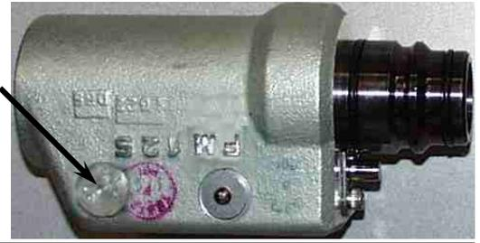
2. Install a 1/4" NPT Hydrostat Fitting into the forward port on the Outlet Body and a Bleed Valve into the rear port on the Outlet Body. These components MUST be installed at the locations shown at right.
