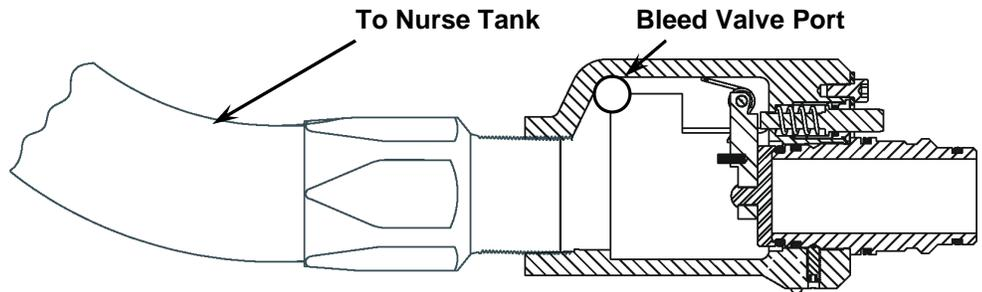
4. Connect the Female (Outlet) Half of the Flo-Max II Coupler to any NH<sub>3</sub> tool bar regulator with the proper hose length. Always place the wrench on the body portion of the coupler when connecting or disconnecting a hose. See FIGURE 5-SAFE INSTALLATION photo on page 5 for minimum parameters for hose length.
