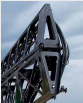
Large Hinge Point W/Self Aligning Plates For More Durability And Longer Life.
