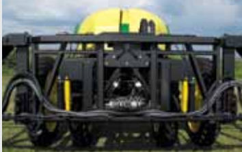
Heavy 6" x 3" Center Section With Ultra Glide Center Pivot Suspension System And Anti-Yah System For Wing Ride.
