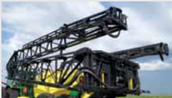
Truss Style Boom With High Tensile Steel
