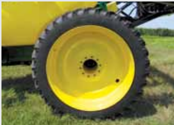
Heavy Duty 10 Bolt Hub, 4 1/2" Spindle On A 5" x 7" x 3/8" Adjustable Axle.
