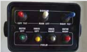
7-Function Hydraulic Control Box Allows For Finger Touch Boom Control On The Seven Self-Returning Toggle Switches.
