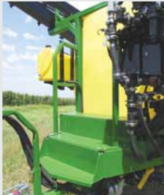
Large Filling Platform And Steps To Access Both Sides Of The Platform.
