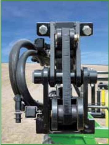
WIDE-BUSHED PINS FOR EXTENDED HINGE LIFE.
