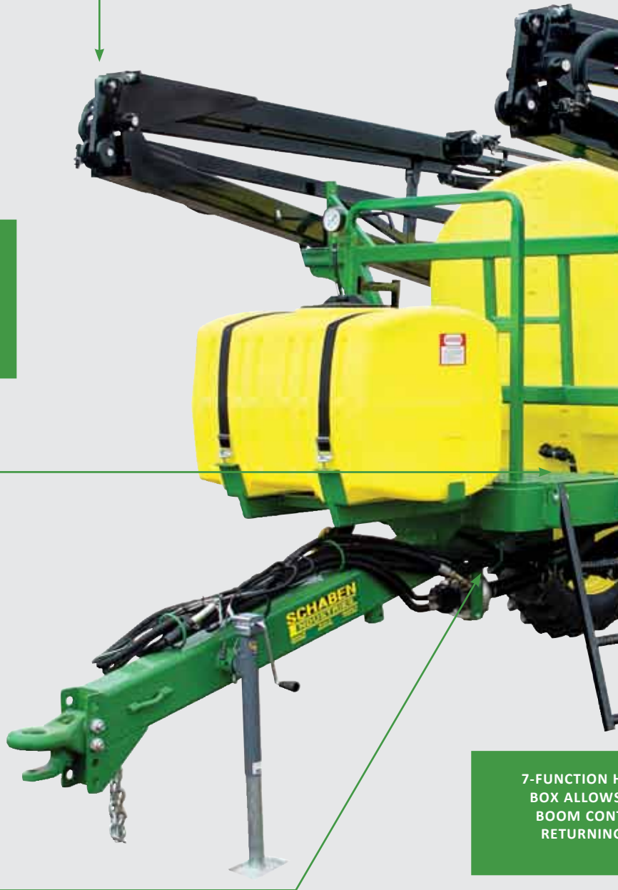
LARGE FILLING PLATFORM WITH STORAGE COMPARTMENT AND STEPS TO ACCESS BOTH SIDES OF THE WALKWAY.
