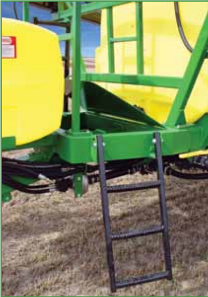
LARGE FILLING PLATFORM WITH STORAGE COMPARTMENT AND STEPS TO ACCESS BOTH SIDES OF THE WALKWAY.
