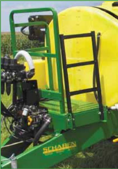
Filling Platform With Steps To Access Tank Lid.
