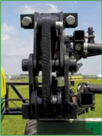
Wide-Bushed Pins For Extended Hinge Life.
