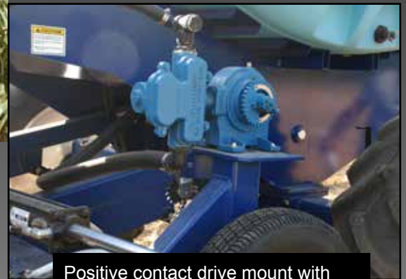
Positive contact drive mount with 155/80R12 tires, John Blue pumps, 2" (5 cm) bottom fill with 2" (5 cm) suction line
