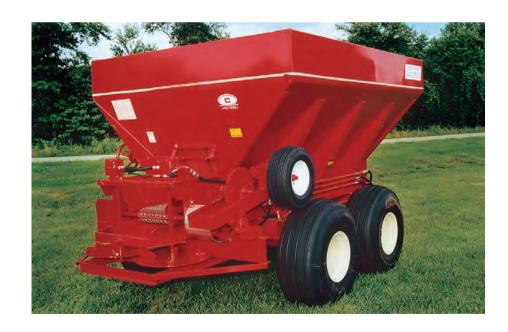
The Chandler Pull-Type Fertilizer Spreader is durable, heavy-duty and well designed for long-lasting, trouble-free service. The design and construction quality of this spreader sets the standard in the agri-business industry. This unit is offered in corrosive-resistant 304 stainless steel. This pull-type spreader has been quality checked and tested to provide the best possible spread pattern for your requirements.
